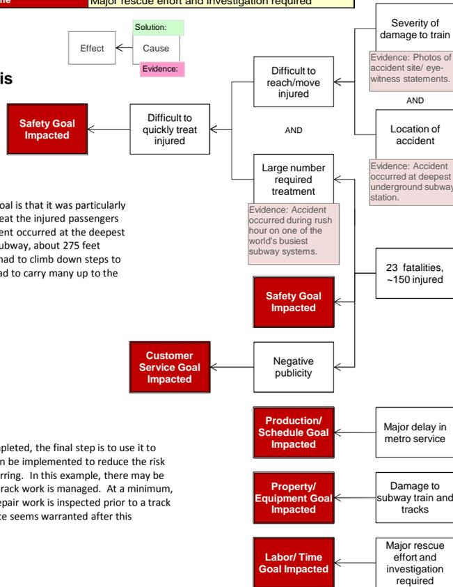
A second impact to the safety goal is that it was particularly difficult to quickly access and treat the injured passengers after the accident. The derailment occurred at the deepest metro station on the Moscow subway, about 275 feet underground. Rescue workers had to climb down steps to reach injured passengers and had to carry many up to the surface.
