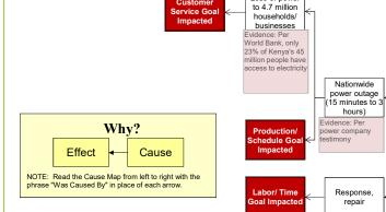
Cause Mapping is a Root Cause Analysis method that captures basic cause-and-effect relationships supported with evidence
